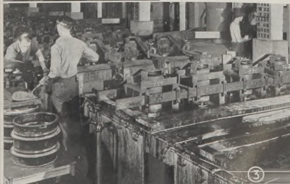
Fig. 3—Solutions in bank of 2000-gallon plating tanks at Cleveland Van der Horst plant are checked and corrected three times daily. In back can be seen battery of rectifier units, each of 2500-ampere capacity, usually four or 10,000 amperes being used per tank
