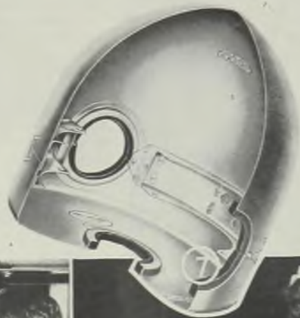
Fig. 6—Fifth step: Cap is gas welded to cone frustum. This requires extremely delicate "touch." Operators wear goggles
