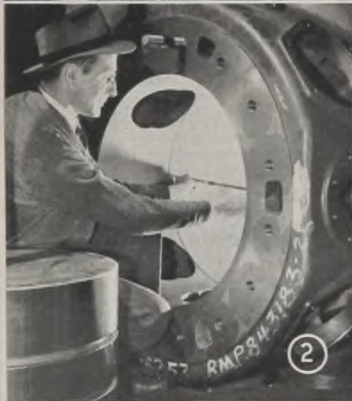
Fig. 1—Navy, Army and Air Forces are employing process widely to reclaim worn radial aircraft and tank engine cylinders such as the one shown here whose surface is being charted on a Brush surface analyzer
