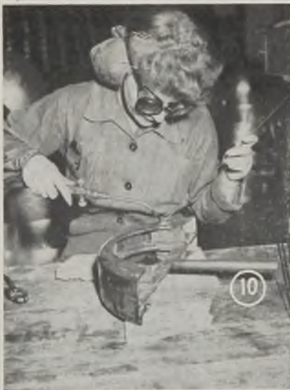
Fig. 8—Sixth step: Now cone with cap in place is stretch-formed to final shape desired
