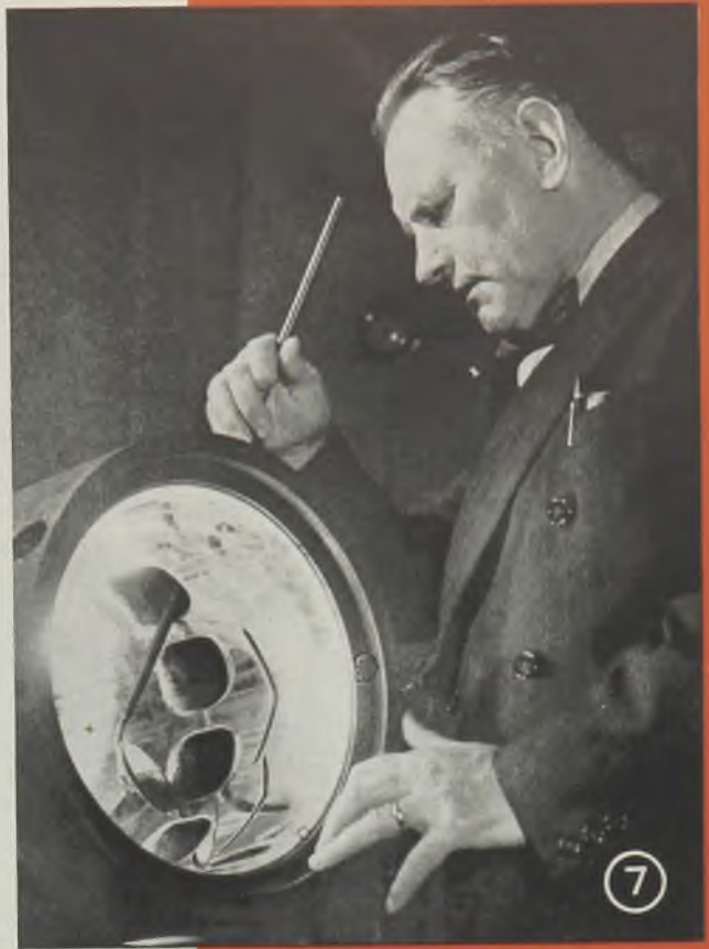
Fig. 7—Hendrich Van der Horst examines cylinder of marine diesel that ran 4¼ million miles on a Dutch ship and has just worn through the Porus-Krome finish
