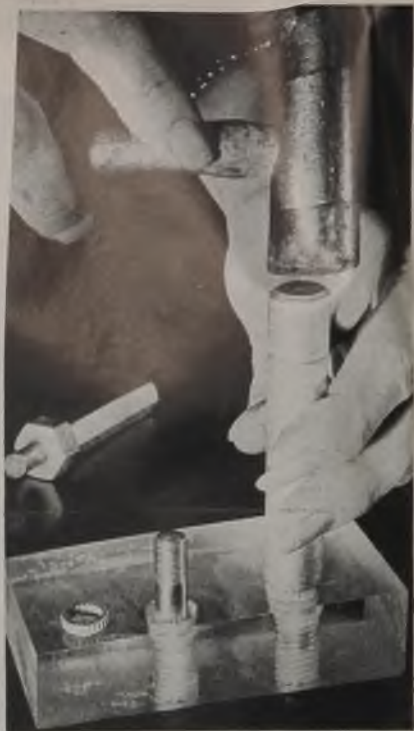
Clear plastic block is used to show system of locking. Stud, center, is locked in place by driving locking ring, left, using hollow driving tool as at right
