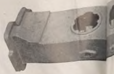
Fig. 5 (Above) — Water-jacketed diesel engine exhaust manifold was fabricated from 1/8-inch sheets
