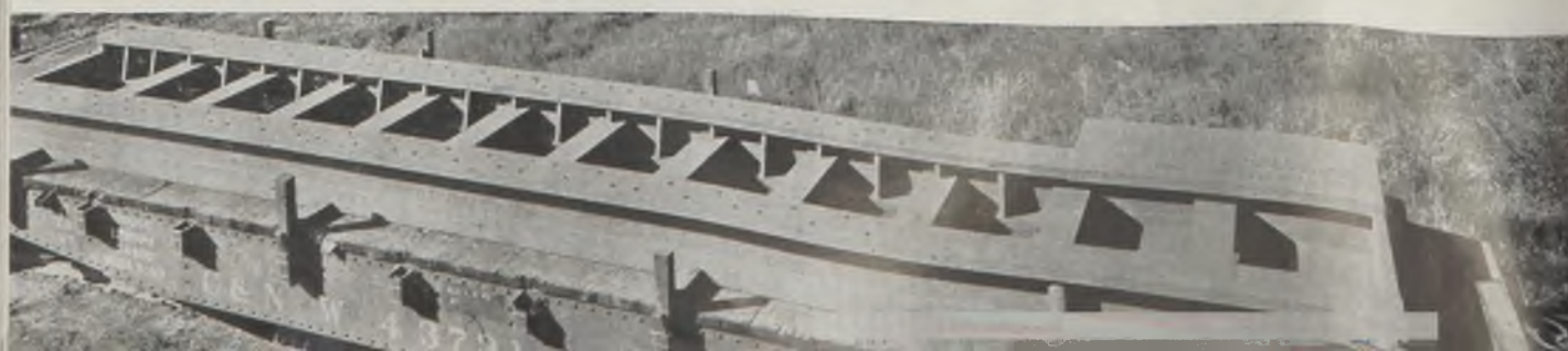
Fig. 3 (Below)—Bed plate for a 38-foot mill roll lathe made up from standard rolled sections
