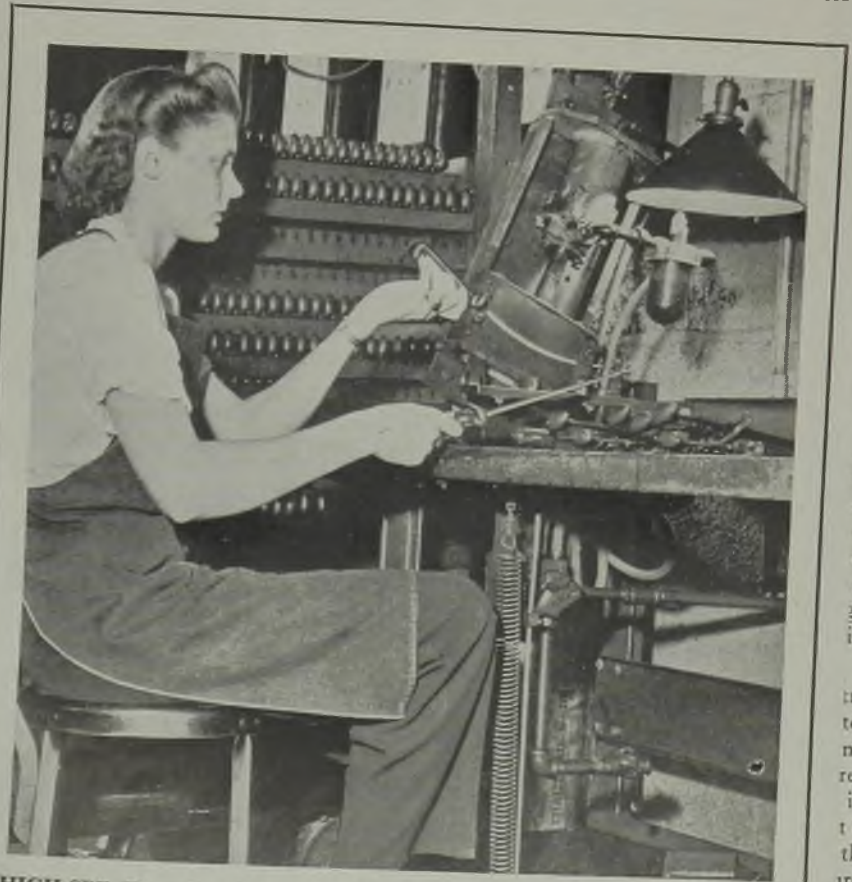
HIGH-SPEED RESILIENCE TEST: —Heat-treated bayonets must withstand a bend both ways to a radius of 18 inches without breaking or taking a permanent set. To match high production rates in its bayonet plant at Ashtabula, O., American Fork & Hoe Co. employs this setup using an air-operated cylinder to compress the blade to the desired curvature between dies as shown. Operator works tester by means of foot controlled valve
