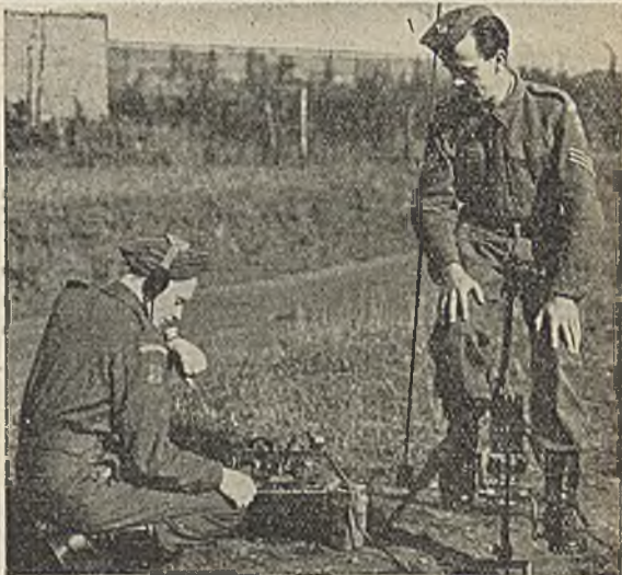
Three more pictures of apparatus designed and delivered for the Army by the radio industry. Top, a portable receiver. Centre, a transmitter-receiver planned for use by patrols in isolated parts. A pedal-driven generator does away with the need for batteries. Below. Mine detectors in action. The enemy has fled. The British wait to advance. A path of safety has to be cleared.
