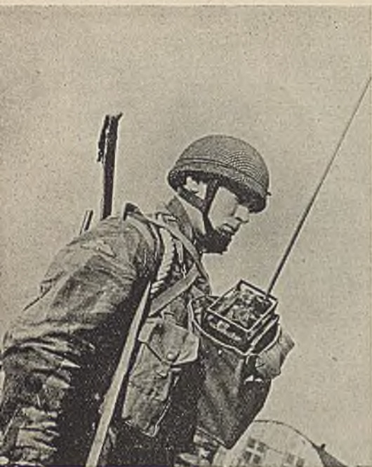
A lightweight portable radio telephone used by Airborne troops. The "38 Set", made in its tens of thousands.
