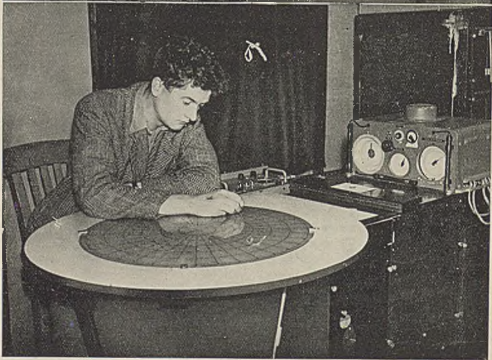
Three pictures of some of the latest Naval radar apparatus. Top left, is a "centimetric" installation for Ack-Ack gunnery. The first operator records elevation, the one in the centre, range, and the one on the extreme right, bearing. Top right, is a lightweight "centimetric" radar warning set. Bottom, the wonderful Skiatron apparatus for tactical plotting.
