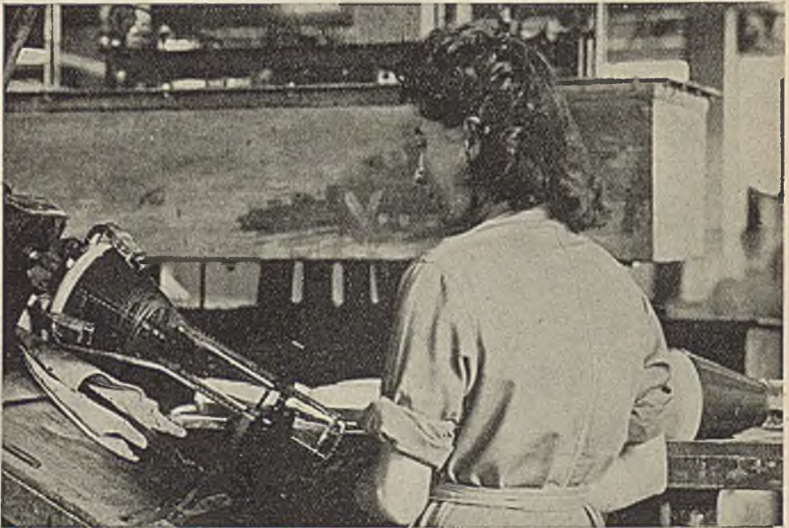
Cathode-ray tube—heart of the radar set. Scores of thousands were made in Britain for equipment of every type. This girl worker is applying a special coating to the inside of a tube.
