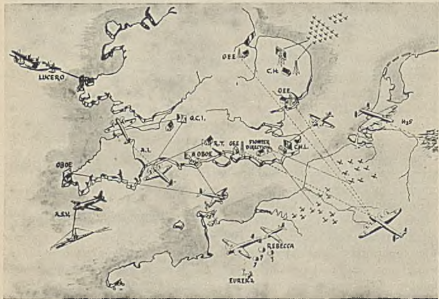
This diagram, prepared by the Ministry of Aircraft Production, shows the uses of many types of radar apparatus, and the names by which the apparatus is known—from C.H., the Chain Home stations which guarded our coasts against surprise attack, to Oboe, which introduced a new and deadly technique of pin-point bombing attack.
