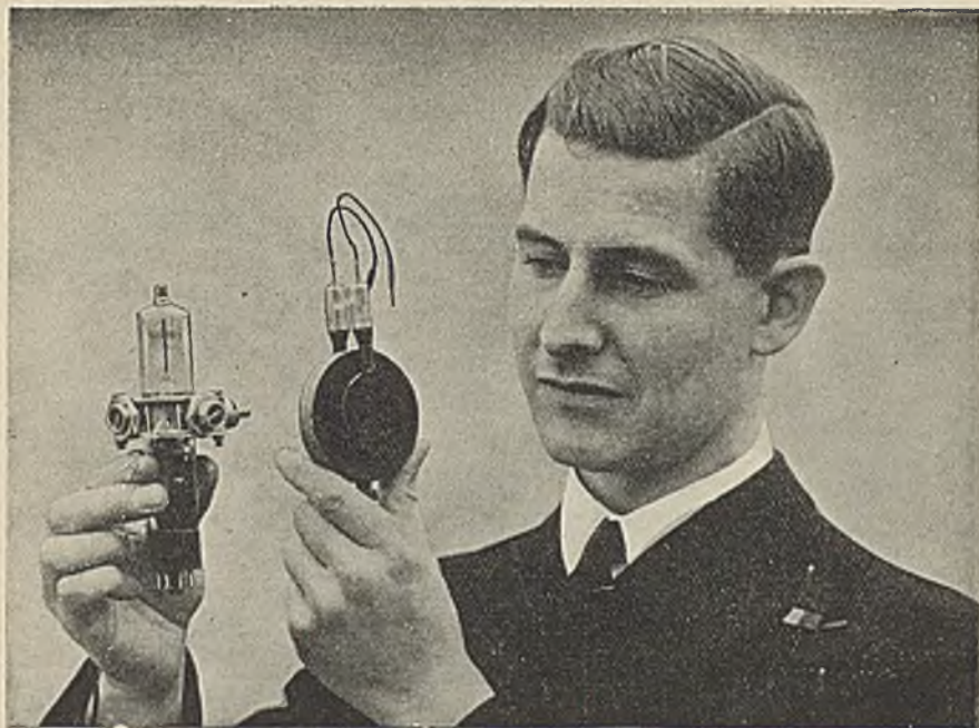
Two valves developed to a high pitch of perfection by British scientists during the war, making centimetre radar possible. Left, the Reflex Klystron and, right, the air-cooled Magnetron.
