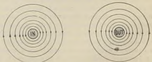
Fig. 13—Lines of Force About Two Conductors Carrying Current in Opposite Directions.
