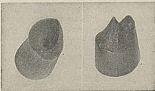
FIG. 30. — Extreme example of cup-and-cone fracture.
