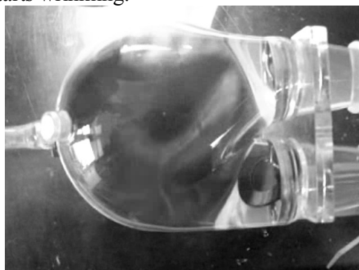
Fig. 3d End of filling – the membrane shape backs to regular, wrinkles dimension decrease.
