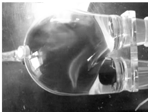
Fig. 3b Beginning of filling – the membrane starts wrinkling.
