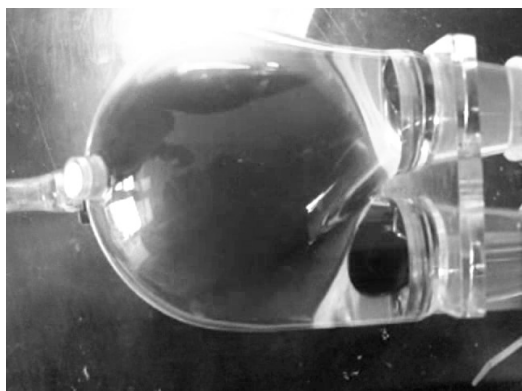
Fig. 8a Full ejection – the membrane is totally displaced and stretched.
