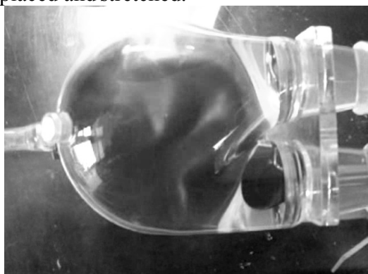
Fig. 3c Filling midpoint – the membrane crosses a mid-plane of chamber (maximal membrane shape distortion).
