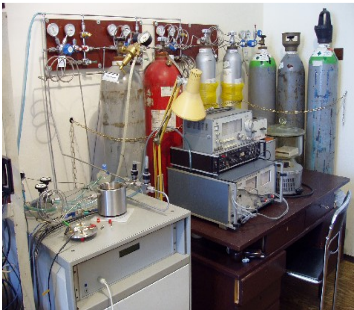
Fig.5. Experimental set-up: measuring chamber with top-cover and gas dosing system.
