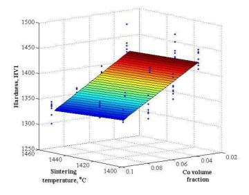
**Figure 27.** Diagram of regression function describing the dependence of hardness on the volumetric share of cobalt and sintering temperature, for the 3-9%Co/97-91%WC\_4 material subjected to sintering and hot isostatic condensation at the temperature of 1425°C in a vacuum furnace
