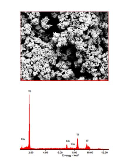
Figure 7. a) Mixture of WC powder (97%), Co powder (3%) after 8 hours of milling in a ball mill, b) Intensity graph as the function of the energy dispersion intensity of X-ray radiation for the WC powder (97%), Co powder (3%) after 8 hours of milling in a ball mill
