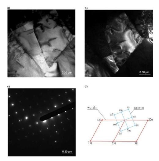
Figure 23. Thin foil structure from WC-Co sintered carbide after sintering at temp. 1460°C;
