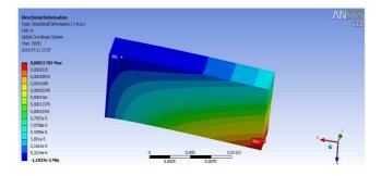
Figure 36. Distribution of the simulated shifts occurring in the cutting edge of a tool consisting of four layers of different share of wolfram carbide and cobalt for the sintering temperature  $T_{sp}=1400^{\circ}C$
