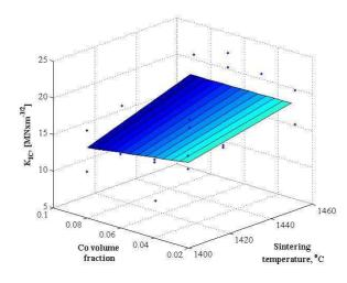
*Figure 30.* Diagram of the regression function describing the dependence of brittle cracking on temperature, and on cobalt share for the 3-9%Co/97-91%WC\_4 material sintered and subjected to hot isostatic condensation at the temperature of 1425°C in a vacuum furnace
