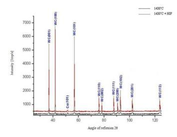
Figure 19. Results of X-ray qualitative phase analysis of tool gradient materials 3-9%Co/97-91WC\_4, sintered in the vacuum furnace at temperature  $T_{sp}$ =1430°C and isostatically condensed at  $T_{sp}$ =1425°C
