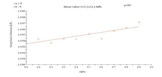
**Figure 34.** Changes of interplanar distance d of the reflex (201) in the function of  $\sin^2 \psi$ , sintering temperature of 1400°C, 3%Co+97%WC
