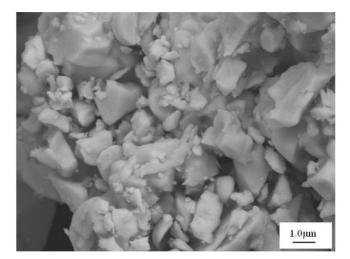
Figure 5. Mixture of WC powder (97%), Co powder (3%) after 8 hours of milling in the ball mill
