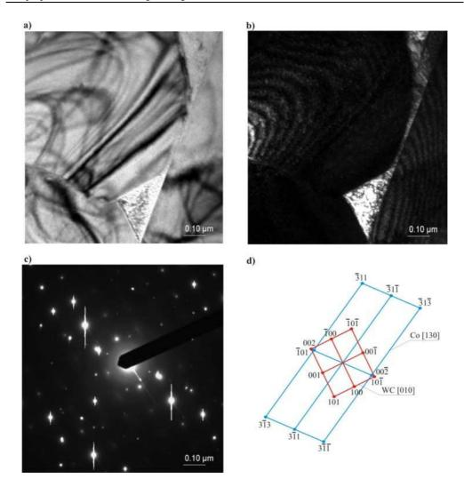
Figure 22. Thin foil structure from WC-Co sintered carbide after sintering at temp. 1460°C;
