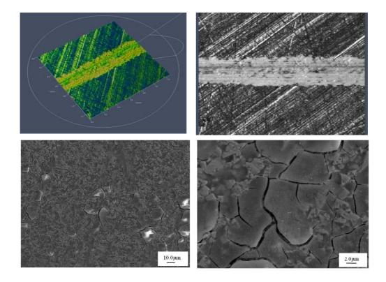
Figure 33. Wear mark of the 3-9%Co/97-91%WC\_4 material sintered in vacuum at the temperature of 1400°C and subjected to isostatic condensation at the temperature of 1425°C after 1000 cycles with the load of 10 N in the base
