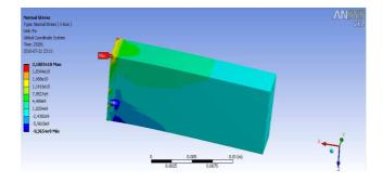
Figure 38. Distribution of the simulated stresses occurring in the cutting edge of a tool consisting of four layers of different share of wolfram carbide and cobalt for the sintering temperature  $T_{sp}=1400^{\circ}C$
