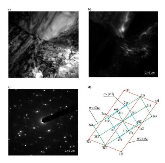
Figure 24. Thin foil structure from WC-Co sintered carbide after sintering at temp. 1400°C;
