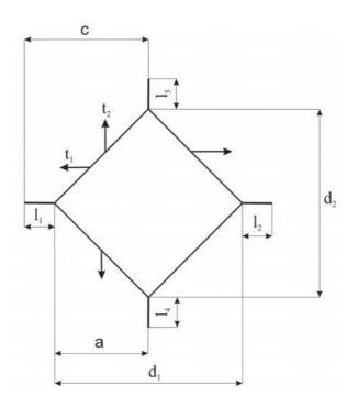
Figure 10. Diagram of the cracking system obtained with Vickers method – Palmqvist method 101 Structure and properties of sintered tool gradient materials
