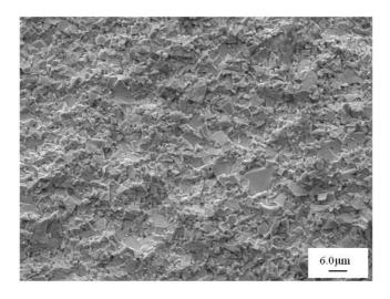
Figure 32. Structure of the fracture of the surface layer of the 3-9%Co/97-91%WC\_4 material sintered in a vacuum furnace at the temperature  $T_{sp}$ =1460°C and subjected to hot isostatic concentration at the temperature  $T_{sp}$ =1425°C in a vacuum furnace
