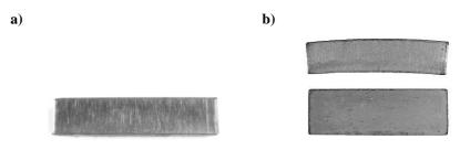
Figure. 6. a) Compact pressed under the pressure of 340MPa from the 3-7%Co/97-73%WC\_5 material, b) cemented tool material 3-7%Co/97-93%WC\_5
