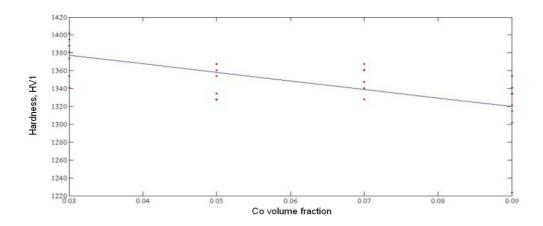
Figure 28. Diagram of regression function describing the dependence of hardness on the volumetric share of cobalt for the 3-9%Co/97-91%WC\_4 material subjected to sintering with hot isostatic condensation at the temperature  $T_{sp}$ =1420°C
