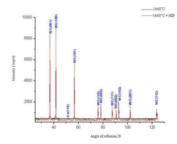
Figure 18. Results of X-ray qualitative phase analysis of tool gradient materials 3-9%Co/97-91WC\_4, sintered in a vacuum furnace at temperature  $T_{sp}$ =1460°C and subjected to isostatic condensation at  $T_{sp}$ =1425°C
