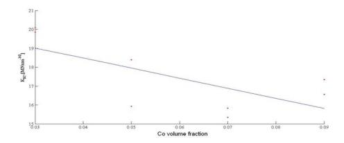
Figure 31. Diagram of the regression function describing the dependence of brittle cracking on the volumetric share of cobalt for the 3-9%Co/97-91%WC\_4 material sintered under the pressure in a vacuum furnace at the temperature  $T_{sp}$ =1420°C
