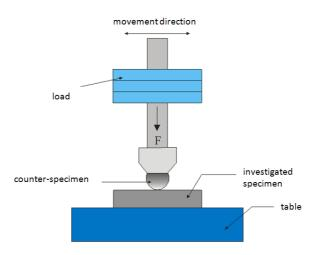
Figure 9. Diagram of the apparatus for testing the resistance to abrasive wear
