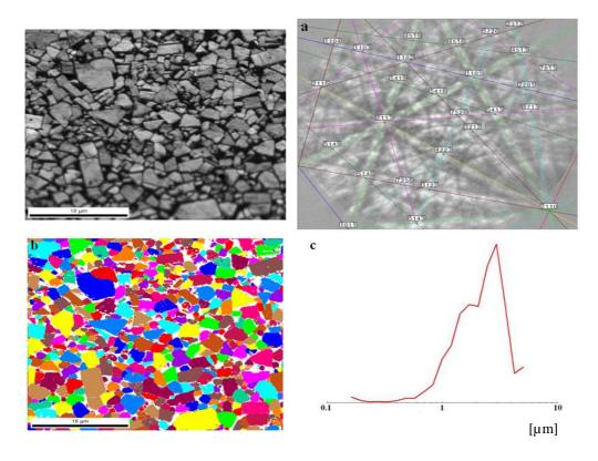
**Figure 21.** Structure of gradient material 3-9%Co/97-91%WC\_4, sintered in the vacuum furnace at temp.  $T_{sp}$ =1400°C and subjected to hot isostatic condensation at temp.  $T_{sp}$ =1425°C, the first layer: a) indexation of the diffraction of the Kikuchi line, b) map of grain size distribution, c) diagram of grain size distribution
