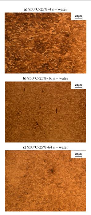
Figure 8. Microstructure evolution of the 26Mn-3Si-3Al-Nb-Ti steel after isothermal holding for time: a) t = 4 s; b) t = 16 s; c) t = 64 s; for the specimens plastically deformed at 900°C,  $\varepsilon = 0.29$
