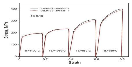
Figure 15. Stress – strain curves for the specimens plastically deformed 4 x 0.19
