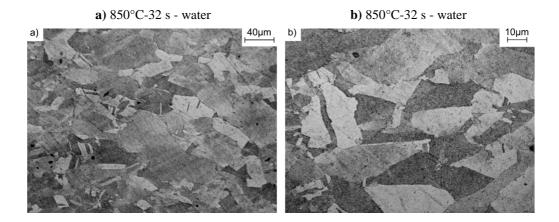
**Figure 21.** Fine, statically recrystallized austenite grains and large statically recovered grains of the steel 27Mn-4Si-2Al-Nb-Ti solution heat-treated from the temperature of 850°C after isothermal holding for 32 s of the specimen compressed with the true strain of 4x0.19 (a, b)
