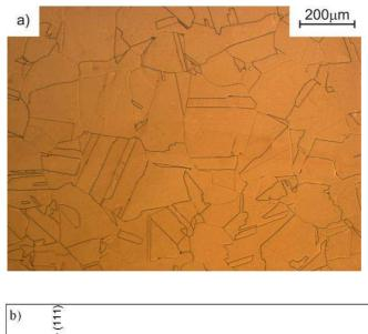
Figure 2. Austenitic microstructure with numerous annealing twins of the 26Mn-3Si-3Al-Nb-Ti steel in the initial state (a) and X-ray diffraction pattern (b)
