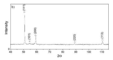
Figure 3. X-ray diffraction pattern (b) and the austenite structure with many annealing twins and parallel  $\varepsilon$  martensite plates of the investigated steel 27Mn-4Si-2Al-Nb-Ti in the initial state (a)
