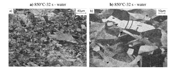
**Figure 19.** Fine, statically recrystallized austenite grains and large statically recovered grains of the steel 27Mn-4Si-2Al-Nb-Ti solution heat-treated from a temperature of 850°C after isothermal holding for 32 s of the specimen compressed with the true strain of 4x0.23 (a, b)
