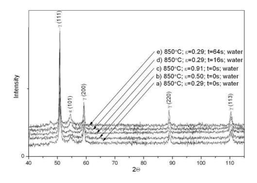
**Figure 10.** X-ray diffraction patterns for 27Mn-4Si-2Al-Nb-Ti steel after various variants of the thermo-mechanical treatment; a) 850°C,  $\varepsilon$ =0.29, t=0 s, b) 850°C,  $\varepsilon$ =0.5, t=0 s, c) 850°C,  $\varepsilon$ =0.91, t=0 s, d) 850°C,  $\varepsilon$ =0.29, t=16 s, e) 850°C,  $\varepsilon$ =0.29, t=64 s
