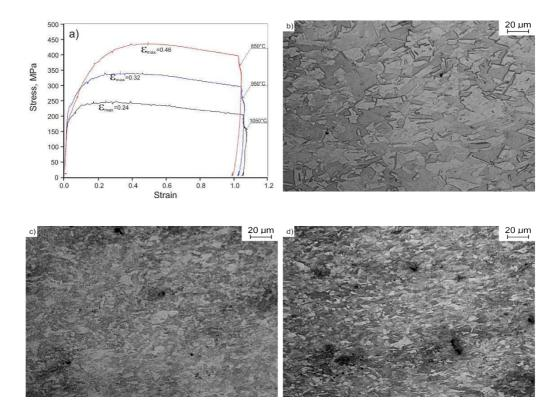
**Figure 7.** Evolution of the microstructure of 26Mn-3Si-3Al-Nb-Ti steel compressed to a various strain: a)  $\sigma$ - $\varepsilon$ curve; b)  $T = 850^{\circ}$ C,  $\varepsilon = 0.23$ ; c)  $T = 850^{\circ}$ C,  $\varepsilon = 0.29$ ; d)  $T = 850^{\circ}$ C,  $\varepsilon = 0.5$
