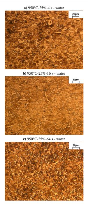
**Figure 9.** Microstructure evolution of the 27Mn-4Si-2Al-Nb-Ti steel after isothermal holding for time: a) t = 4 s; b) t = 16 s; c) t = 64 s; for the specimens plastically deformed at 900°C,  $\varepsilon = 0.29$
