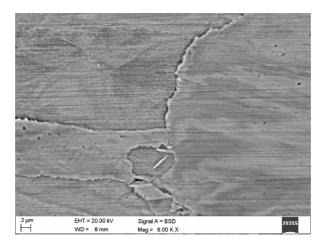
Figure 22. The fine, statically recrystallized grain on jerky-like boundaries of three large, statically recovered grains of the steel 27Mn-4Si-2Al-Nb-Ti solution heat-treated from the temperature of 850°C after isothermal holding for 32 s of the specimen compressed with the true strain of 4x0.19
