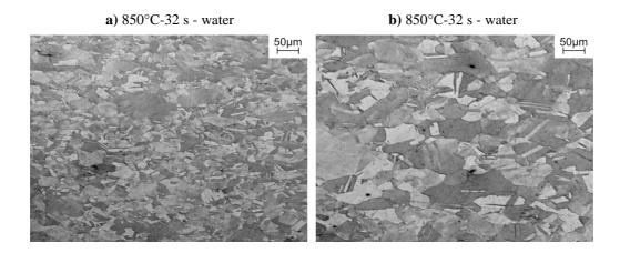
**Figure 25.** Fine, statically recrystallized austenite grains and large statically recovered grains of the 26Mn-3Si-3Al-Nb-Ti steel solution heat-treated from the temperature of 850°C after isothermal holding for 32 s of the specimen compressed with the true strain of 4x0.19 (a, b)
