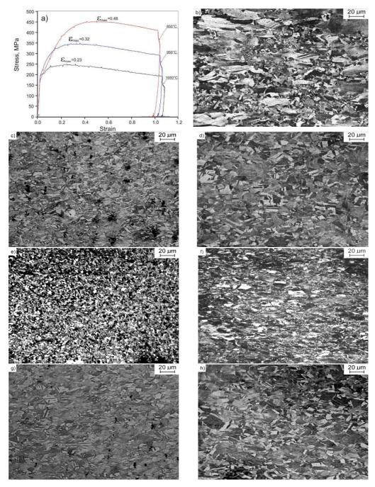
**Figure 6.** Evolution of the microstructure of 27Mn-4Si-2Al-Nb-Ti steel compressed to a various strain: a)  $\sigma$ - $\varepsilon$  curve; b)  $T = 950^{\circ}$ C,  $\varepsilon = 0.5$ ; c)  $T = 950^{\circ}$ C,  $\varepsilon = 0.29$ ; d)  $T = 950^{\circ}$ C,  $\varepsilon = 0.23$ ; e)  $T = 950^{\circ}$ C,  $\varepsilon = 0.91$ ; f)  $T = 850^{\circ}$ C,  $\varepsilon = 0.5$ ; g)  $T = 850^{\circ}$ C,  $\varepsilon = 0.29$ ; h)  $T = 850^{\circ}$ C,  $\varepsilon = 0.23$
