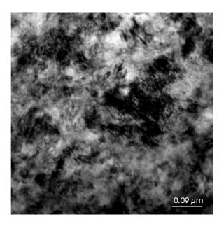
**Figure 20.** Regions of statically recovered austenite with a various dislocation density of the steel 27Mn-4Si-2Al-Nb-Ti solution heat-treated from the temperature of 850°C after isothermal holding for 32 s of the specimen compressed with the true strain of 4x0.23
