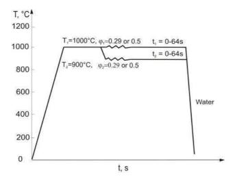
Figure 1. Parameters of the preliminary hot upsetting tests
