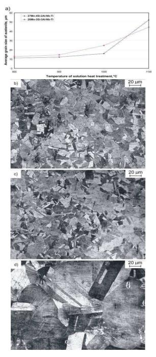
**Figure 4.** Changes of austenite grain size in dependence on temperature (a) and structures obtained after solution heat treatment from a temperature: b) 900°C, c) 1000°C, d) 1100°C; 27Mn-4Si-2Al-Nb-Ti steel
