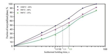
Figure 12. Progress of recrystallization of the 26Mn-3Si-3Al-Nb-Ti steel isothermally held after plastic deformation in various conditions
