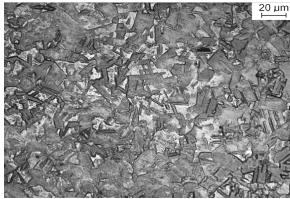
Figure 5. Austenitic structure of the 26Mn-3Si-3Al-Nb-Ti steel after solution heat treatment from a temperature of 900°C
