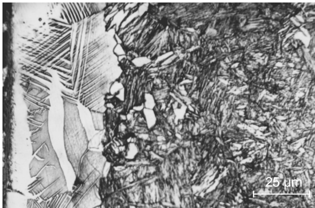
Figure 8. Surface layer microstructure of 38CrAlMo6-10 steel quenched from 920°C, tempered at 575°C and gas-nitrided at 570°C for 8 hrs in an ammonia atmosphere
