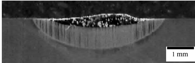
Figure 17. Surface layer of the 32CrMoV12-28 steel after alloying with WC, the laser power of 2.0 kW
