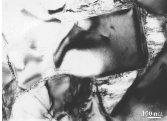
Figure 1. A-type sintered carbide thin foil structure
