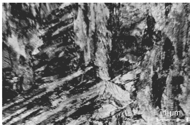
Figure 24. Microstructure of X37CrMoV5-1 steel quenched from 1030°C and tempered at 600°C; thin foil
