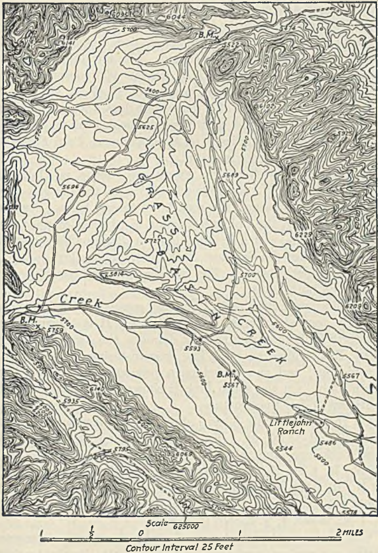
FIG. 12.—Dome with central basin and enclosing escarpment, Grass Creek Basin, Wyoming. (U. S. Geol. Survey.)
