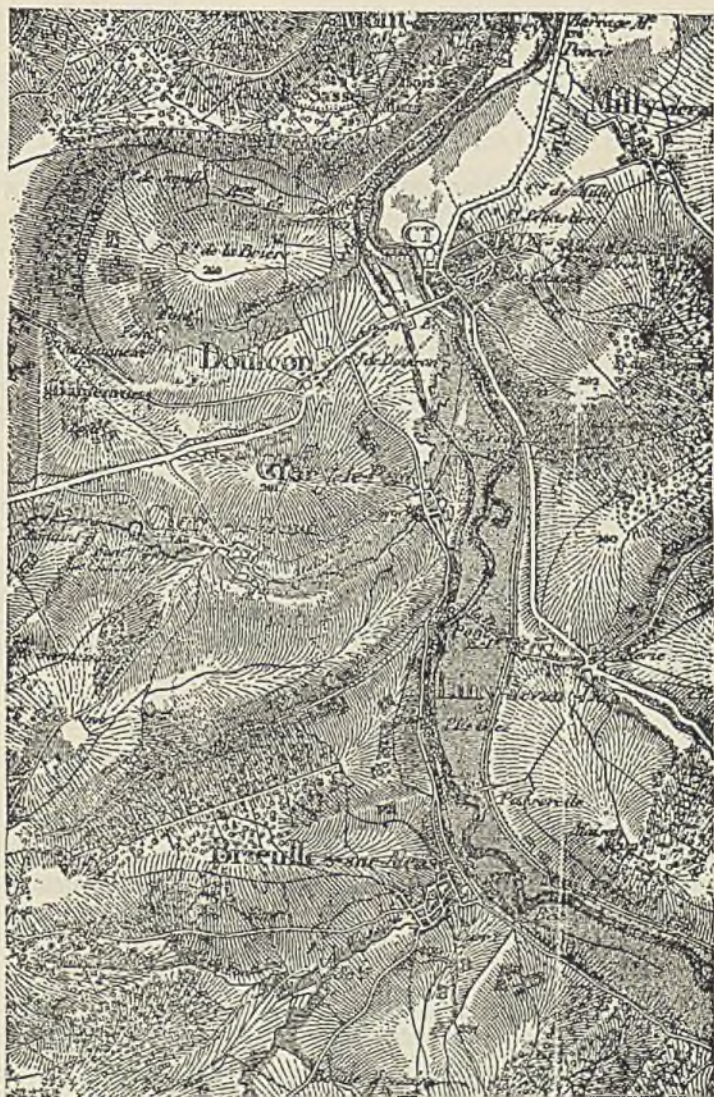
FIG. 1.—Hachures as a method of showing relief. Reproduction of part of Verdun sheet, France.
