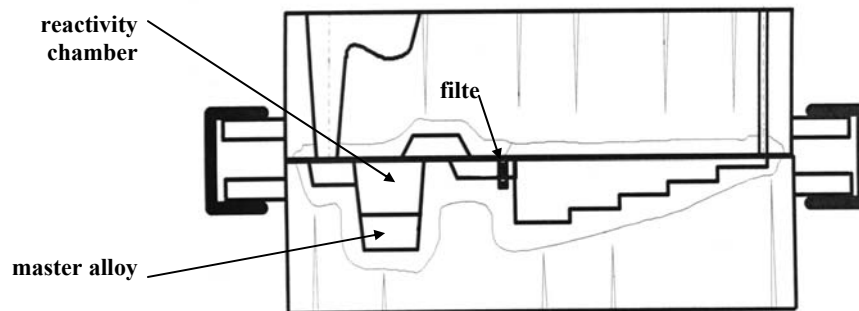
Fig.1. Casting mould with a reaction chamber ready for technological stepped test casting 10, 20, 30, 40 and 50 mm
