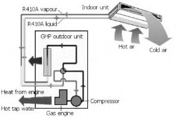
Fig. 9.2 Operation principle of gas heat pump GHP AISIN in cooling mode
