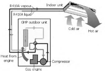
Fig. 9.1 Operation principle of gas heat pump GHP AISIN in heating mode
