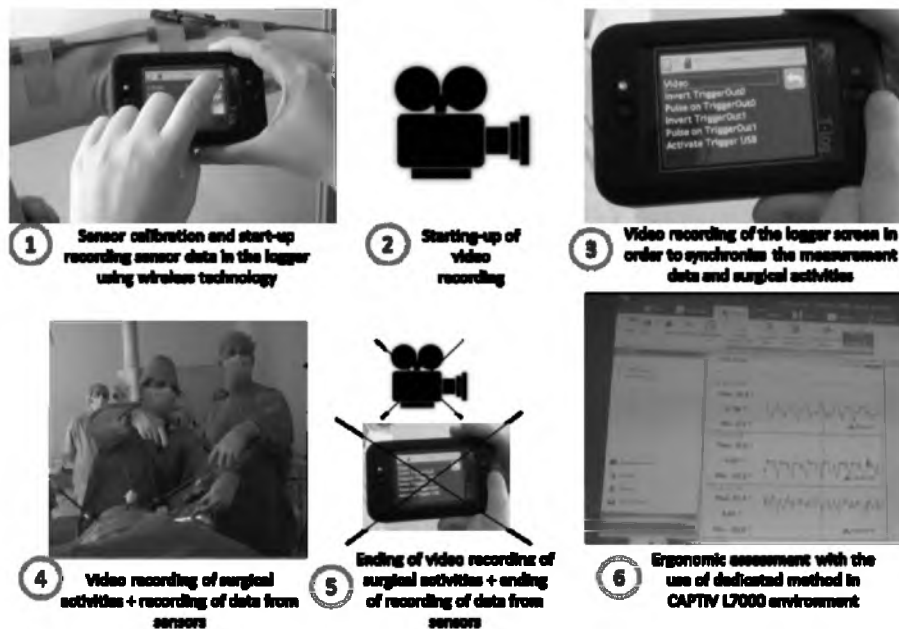
Fig. 1.9 The track of data processing from video recording and measurement recording of surgeon's body position
