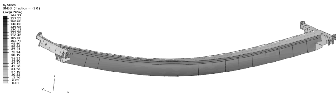
Fig. 7. Reduced stress by Huber-Mises-Hencky theory – the impact of the gravitational force induced by the mass of the structure and mass of the load (5000 [kg])
