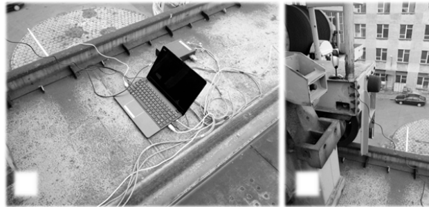
Fig. 6. Measuring circuit for field tests: a) laptop with wi-fi antenna and analogue-to-digital card, b) observation camera
