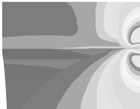
Fig. 6. Results of FEM analysis – contour lines of reduced stresses for congruence coefficient of 0.98
