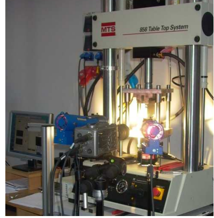
Fig. 5. The test stand for high-speed measurements, Phantom V.9.1. camera and halogen lighting
