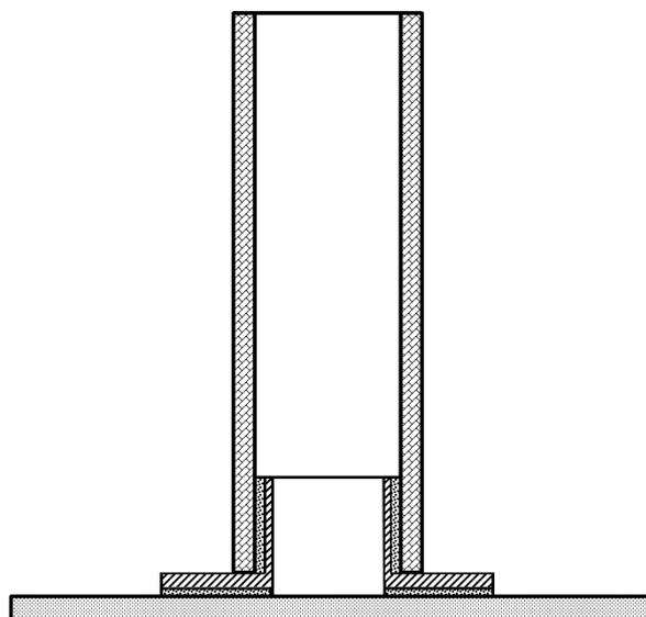
Fig. 3. A scheme of a penetration resistance test rig
