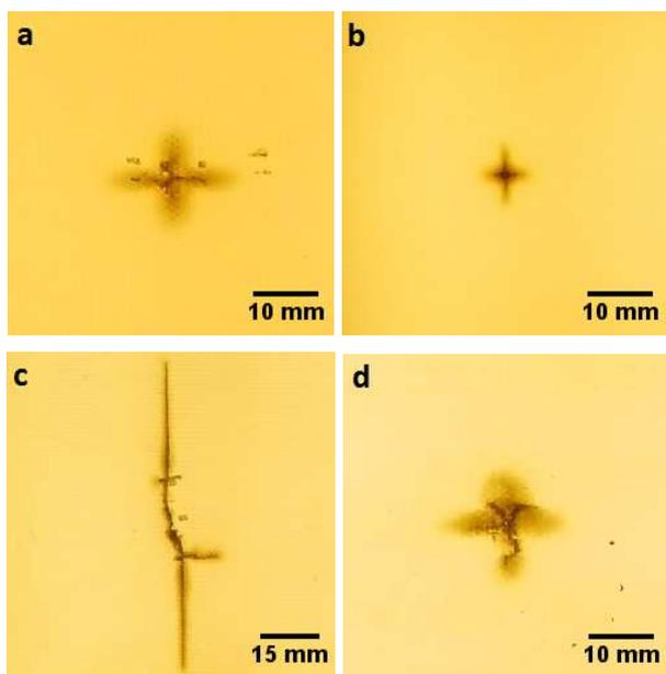
Fig. 2. Exemplary views of the impact damages
