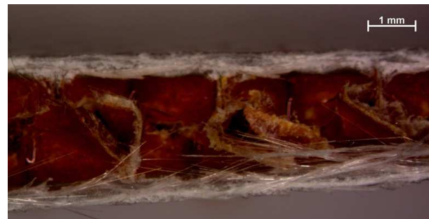
Fig. 8. Shear failure of a core after three-point bending test (magnification 10x)
