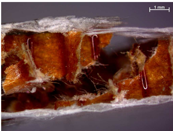
Fig. 4. Failure mode under tensile loading – side view (magnification 10x)
