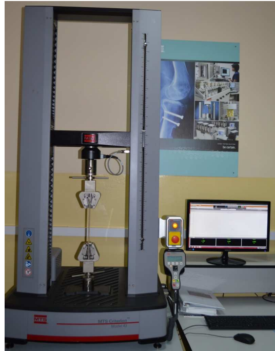
Fig. 1. Experimental setup for tensile tests
