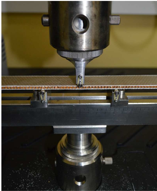
Fig. 6. Experimental setup for three-point bending tests
