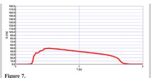
Drainage system discharge hydrogram for increased sewer retention capacity
