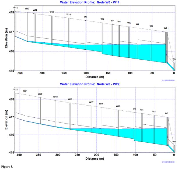
The sewer filling profile after the flow control system was installed and sewer diameters were increased: a) W0-W14, b) W0-W22
