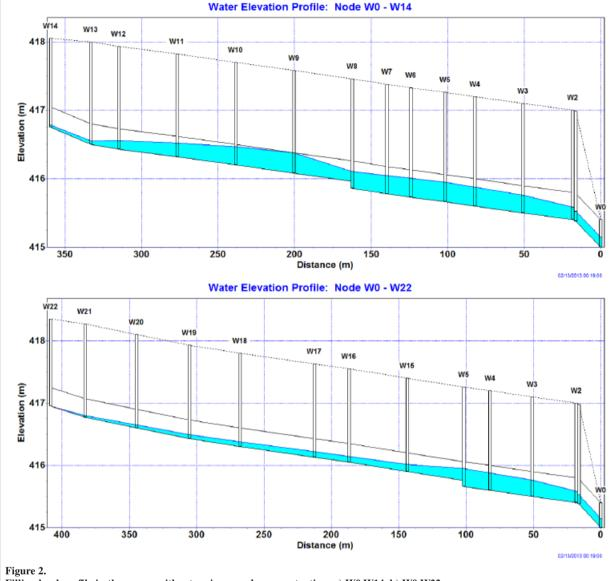
Filling level profile in the sewers without an increased sewer retention: a) W0-W14, b) W0-W22
