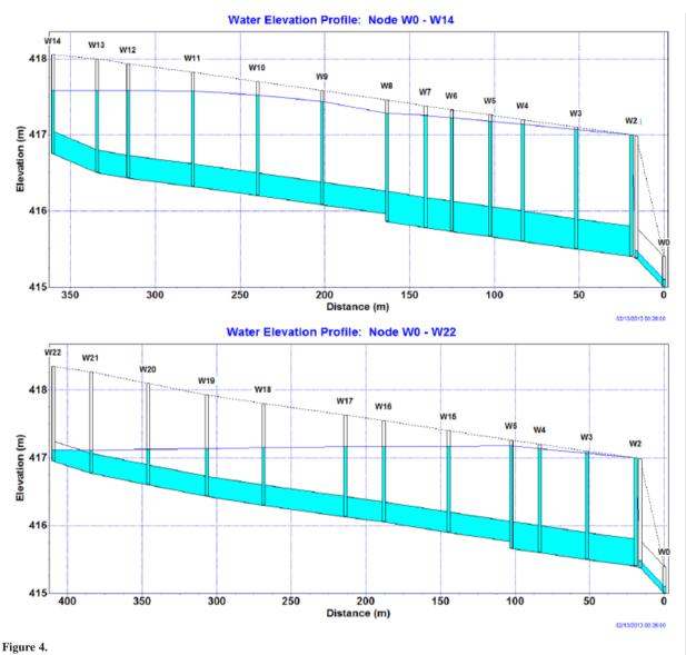
The sewers filling profile after the flow control system was installed: a) W0-W14, b) W0-W22
