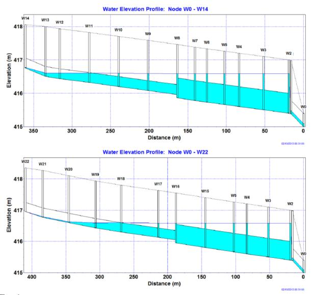
Figure 6. Sewer filling profile for pipes with a Ø600 diameter: a) W0-W14, b) W0-W22
