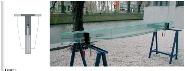
The prototype T-section beam [3]
