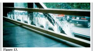
A beam after failure presenting a typical fracture pattern for timber-glass hybrid beam with the web made of annealed float glass [10]
