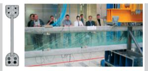
Figure 11. The cross-section of the glass-concrete beam and the specimen during test [9]
