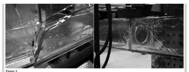
Failure mode of the prototype (left) and crack forming in a 8000 mm long beam (right) [2, 15]
