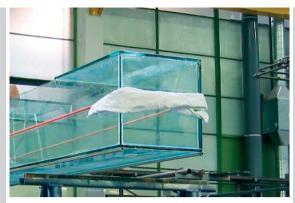
Figure 2. The 4000 mm long prototype with two stainless steel profiles bonded to the bottom plate during lifting process [15]
