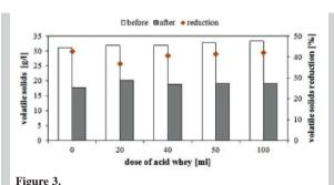
Volatile solids before and after co-digestion process
