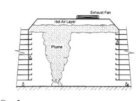
Figure 7. Smoke stratification under a layer of hot air [7]
