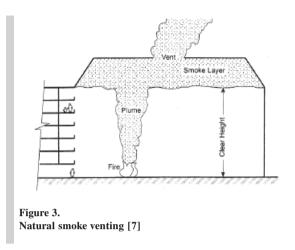
The use of natural ventilation system for the atrium is a good solution. However, it should be appreciated, that there are possible phenomena, the appearance of which can significantly affect the process of smoke exhaust.
