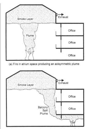
(b) Fire in space open to atrium producing a balcony spill plume
