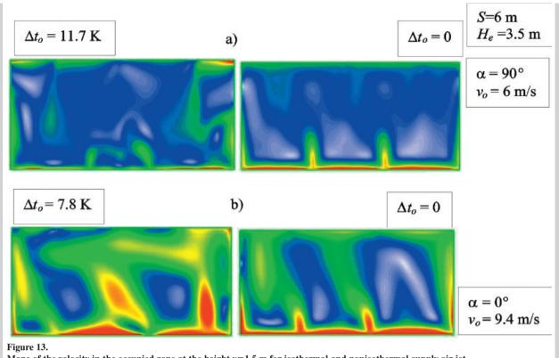
Maps of the velocity in the occupied zone at the height y=1.5 m for isothermal and nonisothermal supply air jet
