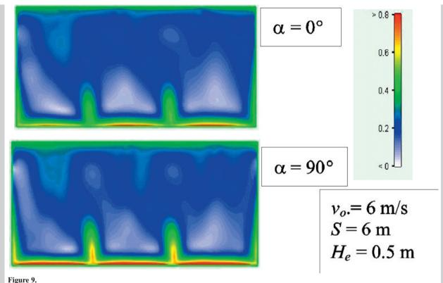
Maps of the velocity in the occupied zone at the height y=1.5 m for various angles of the vanes in the inlets
