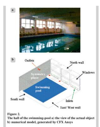
modified, which allowed to deal only with one half of it, assuming that in the other half the airflow is symmetrical. Such a procedure has made it possible to reduce the modelled space and, thus, to refine the discretization grid. Numerical model, after its modification, is to be seen in Fig. 2b. In the numerical cal-
