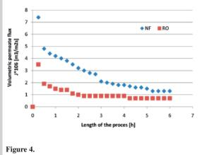
Dependency of the volumetric flux on the length of NF and RO
