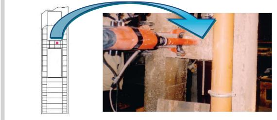
Figure 6. Execution of bore-hole (concrete sample)
