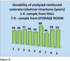
Forecast of service life of analyzed reinforced concrete columns
