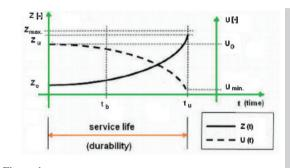
Figure 4. Waste curves Z(t) and usability U(t) of the building structure [6]
