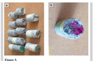
Samples of micro bore-holes taken from tested columns: a) general view, b) phenolphthalein solution coloration
