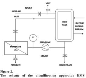
The scheme of the ultrafiltration apparatus KMS Laboratory Cell CF1 (by KOCH)
