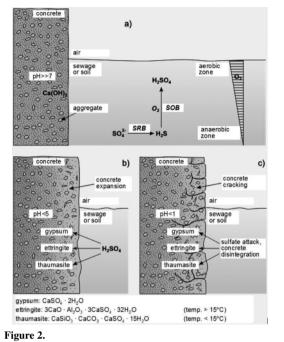
Concrete biodeterioration influenced by sulfate reducing bacteria (SRB) and sulfur oxidizing bacteria (SOB) (picture adapted from [19], with modification)
