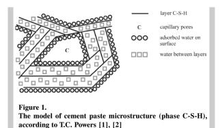
The pores in hardened cement paste are created due to the ratio of ingredients (mainly w/c), method of mixing and consolidation as well as curing conditions.
