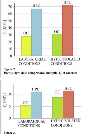
Twenty eight days tensile strength at bending  $(f_{cf})$  of concrete
