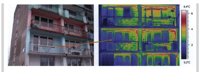
Figure 1. Photo and thermovision picture of the selected partition
