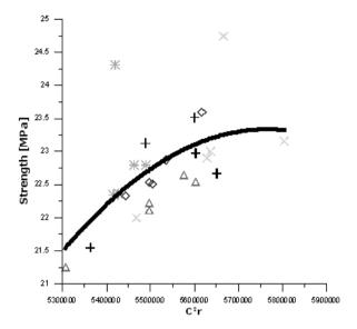
Fig. 2. Relationship between product of the ultrasonic wave velocity and density, and strength: + - speciment no boiling,  $\Diamond$  - speciment after 48 hours of boiling;  $\Delta$  - speciment after 96 hours of boiling; × - speciment after 192 hours of boiling; \* - speciment after 288 hours of boiling
