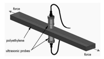
Fig. 1. Scheme of the ultrasonic testing
