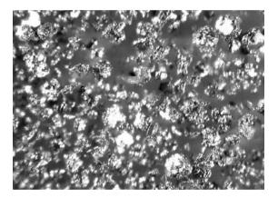
Fig. 2. Iron powder Fe (200) appearance after the chemical silver deposition process; optical microscope, mag. 250x
