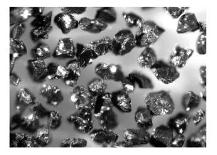
Fig. 3. Glass carbon Cs (100) appearance after the chemical silver deposition processb), optical microscope, mag. 250x
