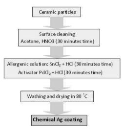
Fig. 1. The stages of the chemical silver coating
