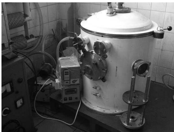
Fig. 1. View of casting area used for degassing and homogenizing composites suspensions [17]
