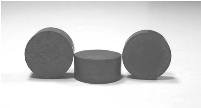
Fig. 1. Composite materials FINEMET ( \text{Fe}_{73.5}\text{Cu}_1\text{Nb}_3\text{Si}_{13.5}\text{B}_9 ) - PEHD
