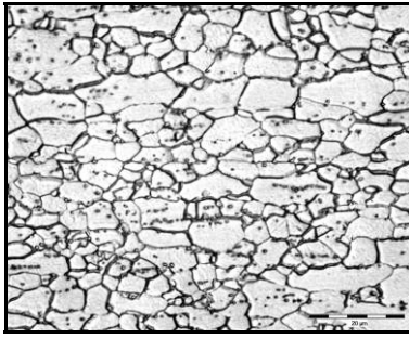
Fig. 18. Microstructure after \varepsilon = 75\% and annealing mode 2
