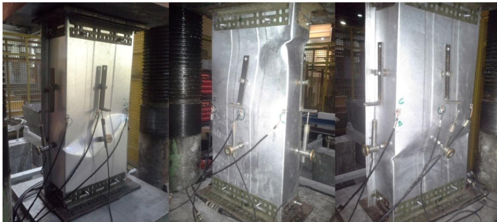
Fig. 32. Straight panels: experimental deformation shapes.
