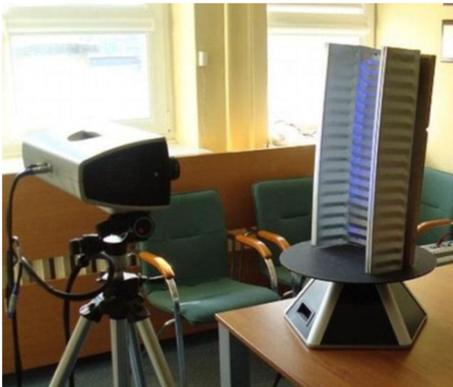
Fig. 15. 3D optical scanning of corrugated panel.
