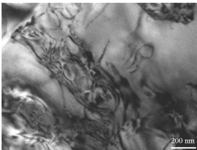
Fig. 5. Structure of sialon substrate, visible numerous dislocations
