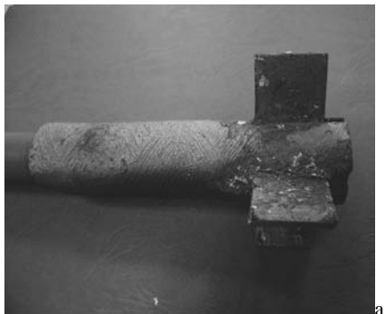
Fig. 21. View of the stirrer: a) after sixteen 30-minute mixing cycles, b) view of the stirrer after clean
