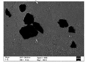
Fig. 27. Scanning electron microscope micrograph of laser modified surface of MCMgAl12Zn1 alloy with Al<sub>2</sub>O<sub>3</sub> particles of the central modified zone, scan rate: 0.5 m/min, laser power: 1.6 kW
