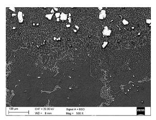
Fig. 24. Scanning electron microscope micrograph of laser modified surface of the MCMgAl9Zn1 alloy with TiC particles at the interface between the modified zone and the substrate, scan rate: 1 m/min, laser power: 1.6 kW
