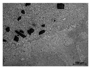
Fig. 21. Border zone of the MCMgAl12Zn1 alloy surface layer after laser treatment with SiC particles, scan rate:  $0.75\,$  m/min, laser power:  $1.6\,$  kW
