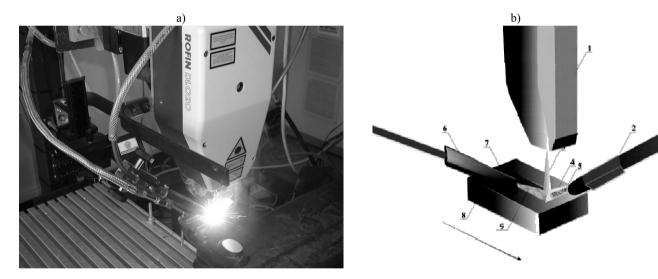
Fig. 1. a) Laser HPDL Rofin DL 020 in working process, b) Laser treatment scheme for casting magnesium alloys: 1 - laser head, 2 - transport gas cylinder and powder feed nozzle, 3 - beam laser, 4 - gas, 5 - powder, 6 - powder feed nozzle, 7 - remelting zone, 8 - base material, 9 - protective gas
