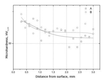
Fig. 42. Cross-section microhardness profile from the MCMgAl6Zn1 substrate with TiC particles, scan rate: 0.75 m/min, laser power: 1.6 kW: A – measurements in the middle run, B – measurements in overlap run
