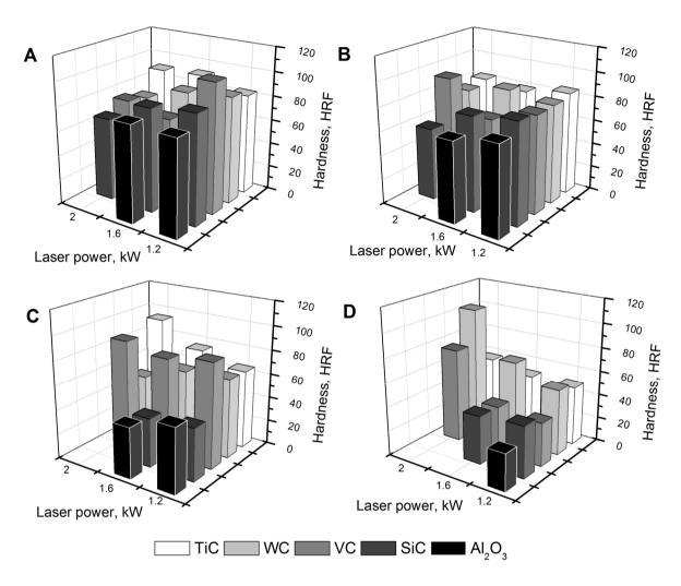
Fig. 34. Change in the average hardness of the surface layer of casting magnesium alloys after laser treatment: A – MCMgAl3Zn1, B – MCMgAl6Zn, C – MCMgAl9Zn1, D – MCMgAl12Zn1
