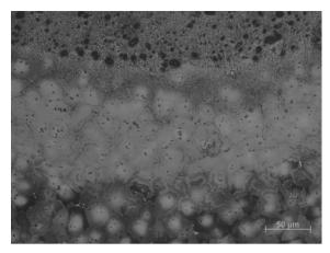
Fig. 18. Structure of the interface between the laser-melted zone, heat affected zone and the substrate of the MCMgAl12Zn1 alloy after laser treatment with WC particles, scan rate: 0.75 m/min, laser power: 2.0 kW
