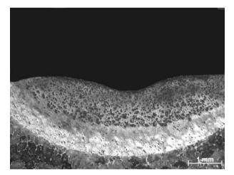
Fig. 13. Surface layer of MCMgAl12Zn1 alloy after laser treatment with TiC particles, scan rate: 0.75 m/min, laser power: 1.6 kW
