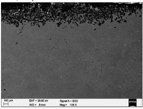
Fig. 26. Scanning electron microscope micrograph of laser modified surface layer of the MCMgAl6Zn1 alloy with SiC particles, scan rate: 0.75 m/min, laser power: 1.6 kW
