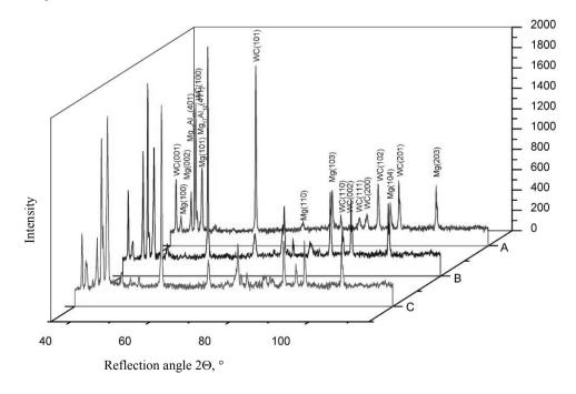
Fig. 32. X-ray diffraction pattern of MCMgAl12Zn1 casting magnesium alloys after laser treatment by tungsten carbide powder, scan rate: 0.7 m/min, laser power: A - 1.2 kW, B - 1.6 kW, C - 2.0 kW
