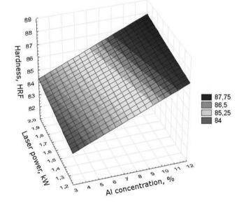
Fig. 37. Simulation of the laser power and aluminium concentration (wt. %) influence on hardness of casting magnesium alloys after laser treatment with WC particles, scan rate 0.75 m/min
