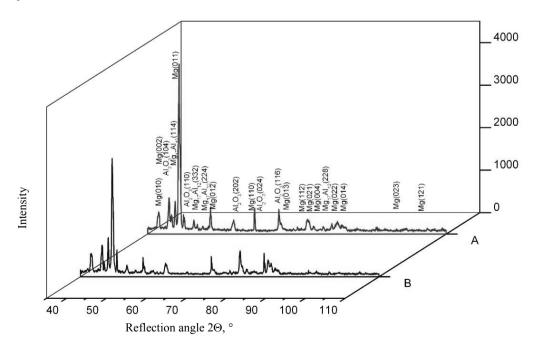
Fig. 30. X-ray diffraction pattern of MCMgAl12Zn1 casting magnesium alloys after laser treatment by aluminium oxide powder, scan rate: 0.75 m/min, laser power: A - 2.0 kW, B - 1.6 kW
