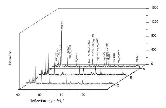
Fig. 33. X-ray diffraction pattern of MCMgAl12Zn1 casting magnesium alloys after laser treatment by titanium carbide powder, scan rate: 0.75 m/min, laser power: A – 1.2 kW, B – 1.6 kW, C – 2.0 kW
