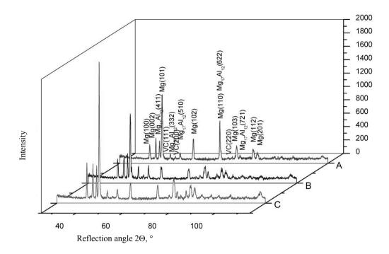
Fig. 31. X-ray diffraction pattern of MCMgAl12Zn1 casting magnesium alloys after laser treatment by vanadium carbide powder, scan rate: 0.75 m/min, laser power: A - 1.2 kW, B - 1.6 kW, C - 2.0 kW
