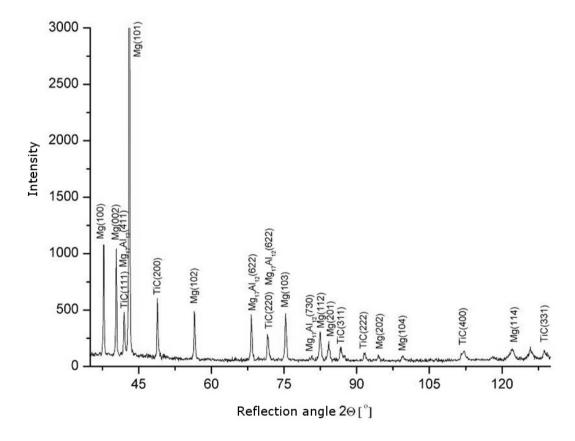
Fig. 44. X-ray diffraction pattern of the MCMgAl6Zn1 casting magnesium alloy after laser treatment with TiC particles, scan rate: 0.75 m/min, laser power: 1.6 kW
