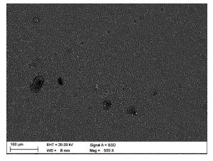
Fig. 28. Scanning electron microscope micrograph of laser modified surface of MCMgAl12Zn1 alloy with VC particles of the central modified zone, scan rate: 0.75 m/min, laser power: 1.6 kW
