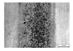
Fig. 11. View of the MCMgAl12Zn1 casting magnesium alloy face of weld after laser treatment with Al<sub>2</sub>O<sub>3</sub>, scan rate: 0.5 m/min, laser power: 2.0 kW
