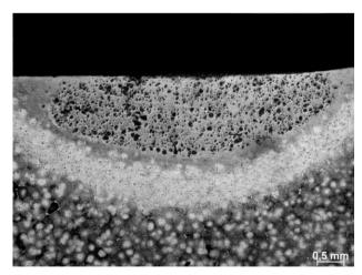
Fig. 14. Surface layer of MCMgAl9Zn1 alloy after laser treatment with WC particles, scan rate: 0.75 m/min, laser power: 2.0 kW
