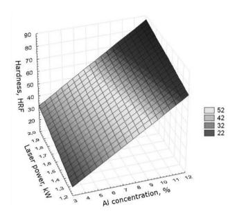
Fig. 39. Simulation of the laser power and aluminium concentration (wt. %) influence on hardness of casting magnesium alloys after laser treatment with Al<sub>2</sub>O<sub>3</sub> particles, scan rate 0.5 m/min
