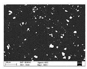
Fig. 23. Scanning electron microscope micrograph of laser modified surface of MCMgAl3Zn1 alloy with TiC particles of the central modified zone, scan rate: 0.75 m/min, laser power: 1.2 kW
