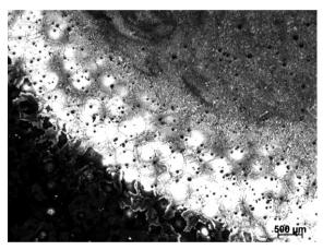
Fig. 20. Remelting path edge of the MCMgAl9Zn1 alloy surface layer after laser treatment with WC particles, scan rate: 0.75 m/min, laser power: 2.0 kW
