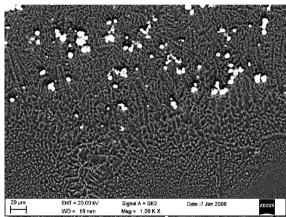
Fig. 25. Scanning electron microscope micrograph of laser modified surface of the MCMgAl6Zn1 alloy with WC particles at the interface between the modified zone and the substrate, scan rate: 0.5 m/min, laser power: 1.6 kW
