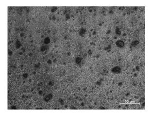
Fig. 19. Central zone of the MCMgAl12Zn1 alloy surface layer after laser treatment with WC particles, scan rate: 0.75 m/min, laser power: 2.0 kW
