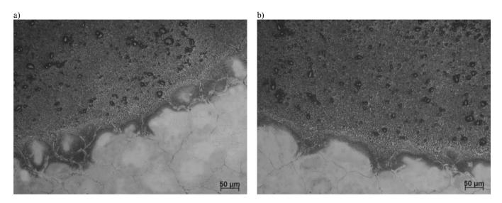
Fig. 43. Boundary between alloyed zone and heat affected zone of MCMgAl6Zn1 alloy after laser treatment with TiC particles, scan rate: 0.75 m/min, laser power: 1.6 kW
