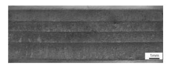
Fig. 40. View of the MCMgAl6Zn1 casting magnesium alloy face of weld after laser treatment with TiC, scan rate: 0.75 m/min, laser power: 1.6 kW
