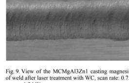
Fig. 9. View of the MCMgAl3Zn1 casting magnesium alloy face of weld after laser treatment with WC, scan rate: 0.75 m/min, laser power: 1.2 kW
