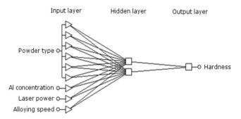
Fig. 2. Scheme of MLP neural network calculates hardness
