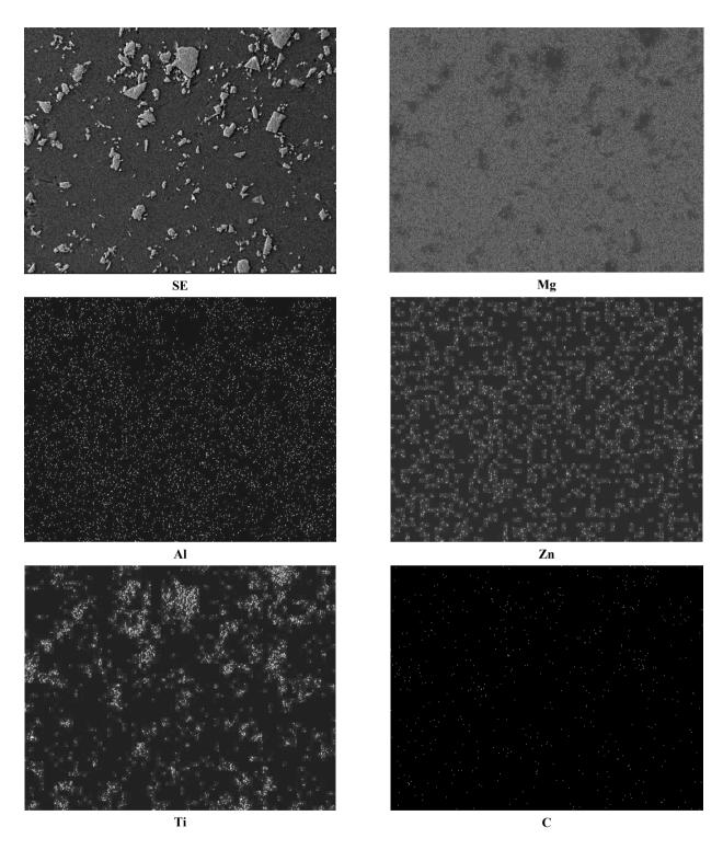
Fig. 45. X-ray mapping of the microstructure MCMgAl6Zn1 cladding layer and the distribution of Mg, Al, Zn, Ti, C, scan rate: 0.75 m/min, laser power: 1.6 kW
