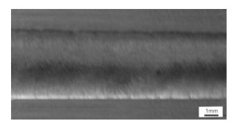
Fig. 8. View of the MCMgAl12Zn1 casting magnesium alloy face of weld after laser treatment with TiC, scan rate: 0.75 m/min, laser power: 1.2 kW
