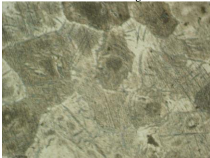
Rys. 6. Struktura staliwa FeAl6, ferryt + perlit, x50 Fig. 6. FeAl6 cast steel microstructure, ferrite + pearlite, mag. 50
