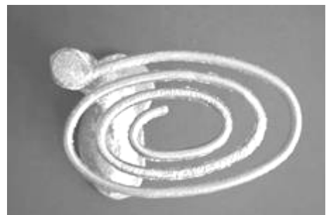
Fig. 10. Spiral test at 1600°C
