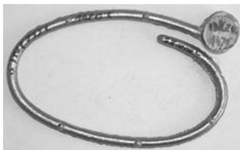
Fig. 7. Spiral test at 1420°C
