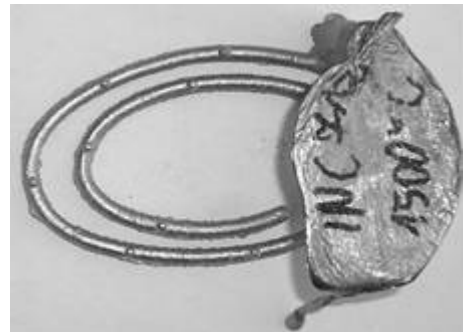
Fig. 9. Spiral test at 1500°C
