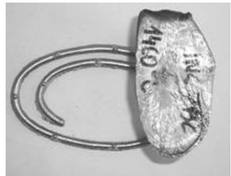
Fig. 8. Spiral test at 1460°C
