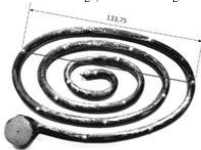
Fig. 12. Method of shrinkage measurement in the casting of fluidity spiral
