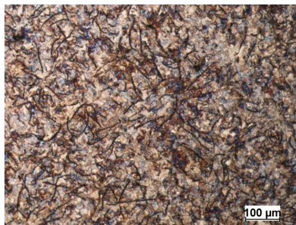
Fig. 10. Cast iron W6synth (FeSi75) matrix
