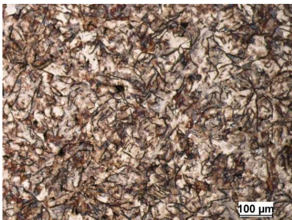
Fig. 11. Cast iron W7pig (FeSi75) matrix
