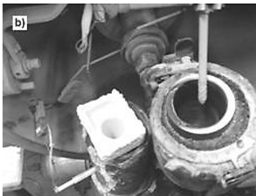
Fig. 2. Balzers VSG-02 VIM furnace chamber
