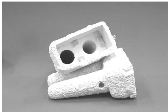
Fig. 1. Ceramic moulds with visible „blue” and “white” canals
