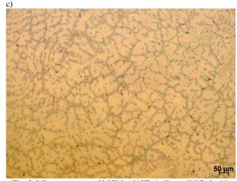
Fig. 2. Microstructures of MCMgAl12Zn1 alloy solidified with cooling rate: a) 0.6°C/s, b) 1.2°C/s, c) 2.4°C/s. Magnification 100x.
