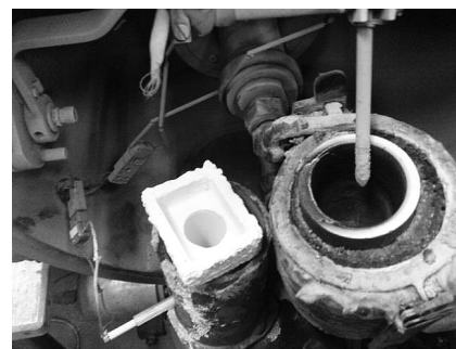
Fig. 3. Chamber of VSG-02 induction furnace
