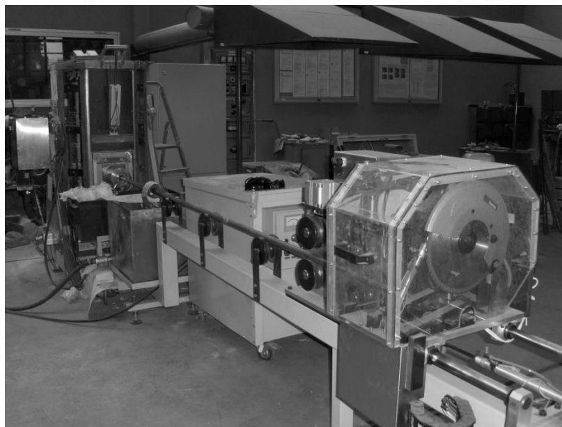
Fig. 1. Scheme (a) and view (b) of stand of horizontal continuous casting: 1 – induction furnace (tundish), 2 – continuous casting mould, 3 – system of recooling, 4 – system of ingot drawing, 5 – system of ingot cutting
